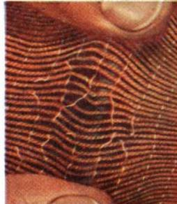
**3** Most tire cords are bunched and gapped by slender cross threads. Weak spots, "slacker cords", overworked cords result. BFG cords, instead, are sealed in live rubber, with uniform spacing and tension.
